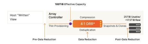
Figure 1. Block storage service effective used capacity example
