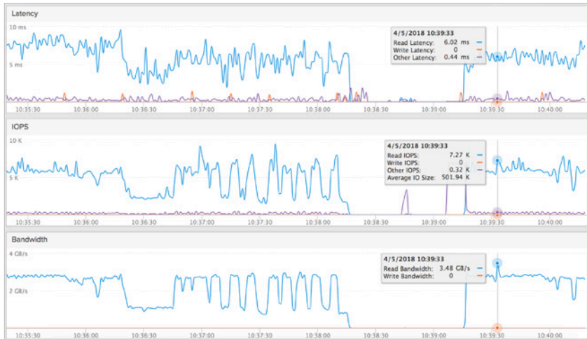
FIGURE 6. Screenshot taken from the FlashBlade UI while training a ResNet-50 model. The storage bandwidth, shown in the bottom graph, indicates an aggregate demand of nearly 3.5 GB/s. The brief dip in bandwidth indicates the input pipeline is filled with images waiting on GPUs to process.
