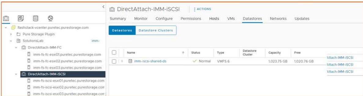
FIGURE 8 View of datastores within vSphere cluster for iSCSI service profiles
