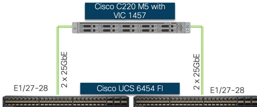
Figure 16 Cisco UCS C220 M5 to Cisco UCS 6454 FI Connectivity
