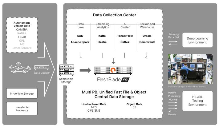
Multiple application types can be run, from data lakes to data warehouses, on a single unified fast file and object platform, which allows everything from ingest to training simulation and testing to be completed on a centralized platform. It simplifies deployment, adapts to change, increases quality, and reduces time to market.
