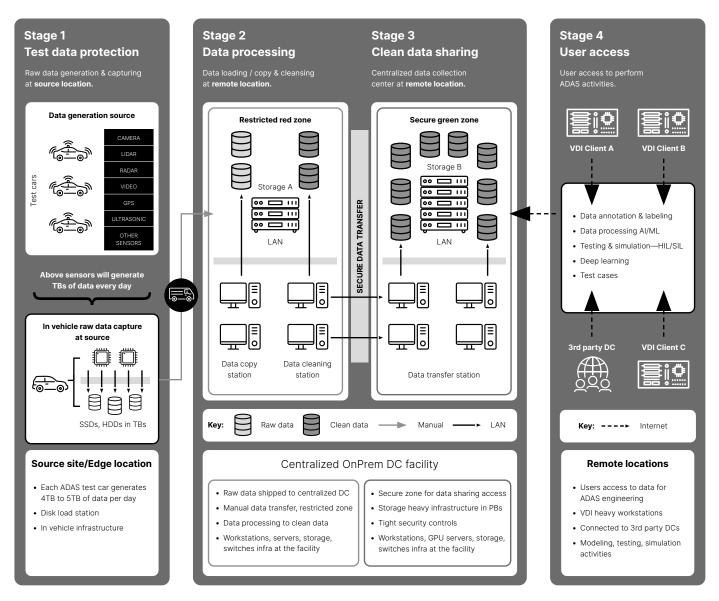
To enable feature development and training, data is ingested from a vehicle, stored for labeling and then processed through a test suite. The defined rules are applied, and testing and validation is carried out before deploying the model back to the vehicle. And that cycle is repeated.
