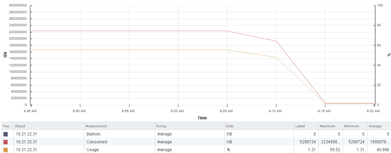
Figure 17: Single ESXi host memory utilization during 100 MCS Knowledge Worker simulation showing no ballooning or swapping and a maximum of 55.5% memory used during the simulation
