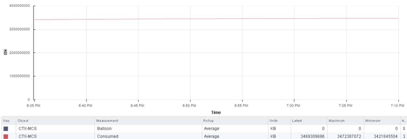
Figure 43: 16 host ESXi cluster consistent memory utilization during 1600 Knowledge worker Login VSI simulation
