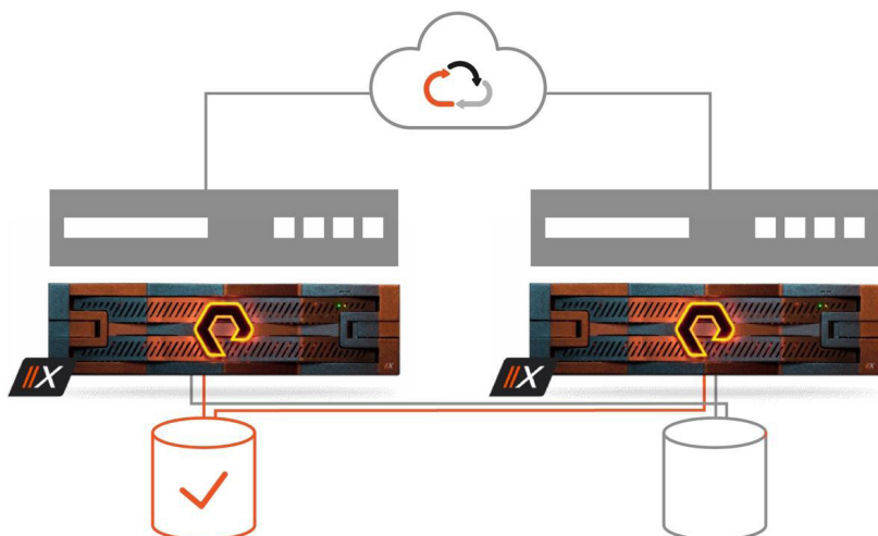
FIGURE 3 Pure1 and ActiveCluster architecture: Pure1 mediates between clustered FlashArray systems to provide high availability for SQL Server
