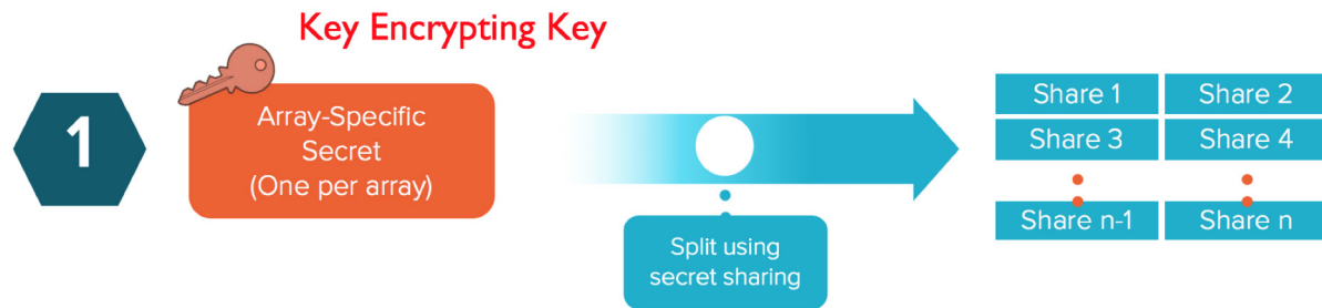
FIGURE 1. Array key generation
