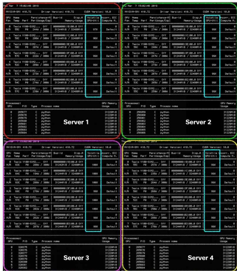
FIGURE 17. FULL GPU UTILIZATION ACHIEVED DURING MULTIPLE-NODE TESTS
