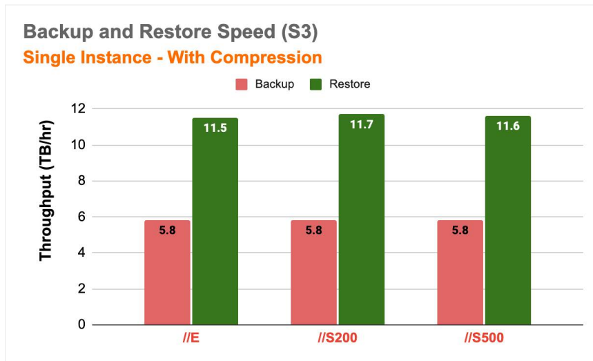
FIGURE 6 Summary of single database evaluation using S3 (With Compression)
