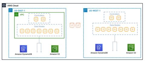
Pure Cloud Block Store performs asynchronous replication to multiple Regions in multiple AZs.
