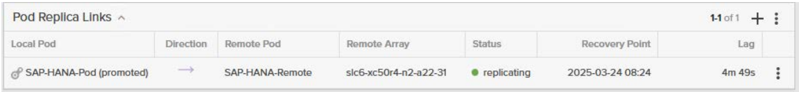
FIGURE 20 Monitoring the pod replica link status on the secondary site's FlashArray.
