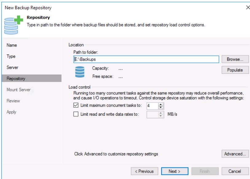
Figure 18: Location and load control configuration
